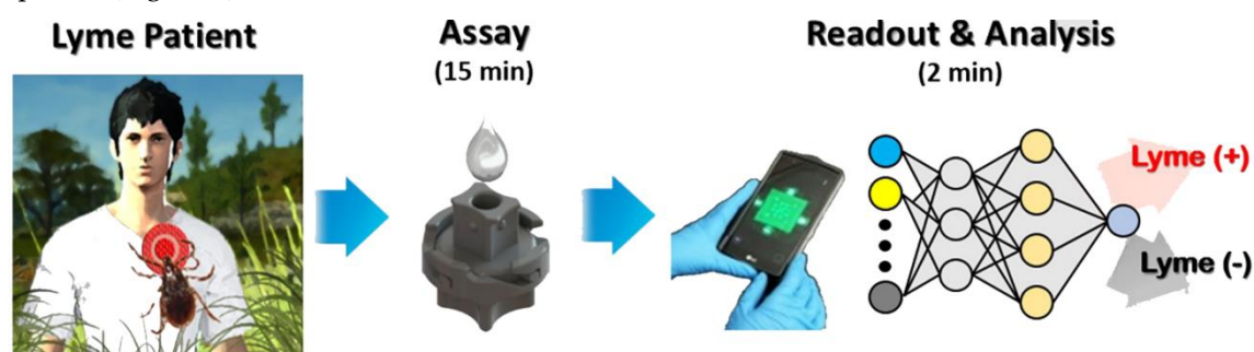
Figure 4. Sequential steps of the devised method to detect Lyme disease using a mobile phone to capture the image, and employing a DL approach to analyze the data to determine the test result 31 . Reproduced with permission from H.-A. Joung, Z. S. Ballard, J. Wu, D. K. Tseng, H. Teshome, L. Zhang, E. J. Horn, P.
